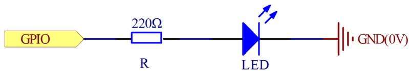
As shown in the schematic diagram above, the anode of LED is connected to Arduino's GPIO via a resistor, and the cathode of LED is connected to the ground(GND). When the GPIO output high level, the LED is on; when the GPIO output low level, the LED is off.
