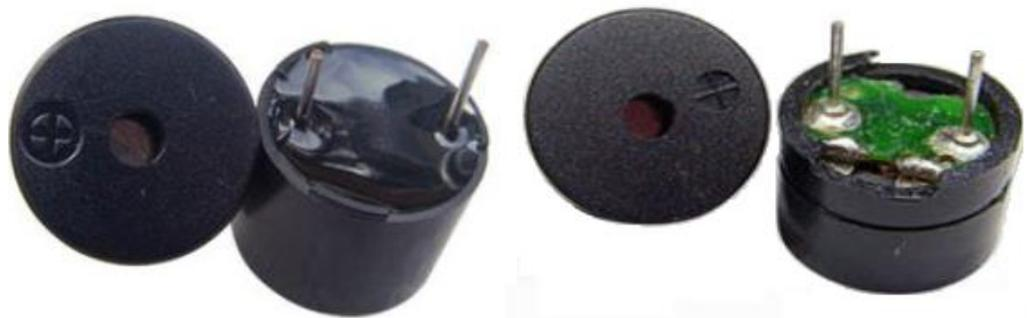
When you place the pins of buzzers upward, you can see that two buzzers are different, and the buzzer on the green circuit board is the passive buzzer. In this study, the buzzer we used is an active buzzer. An active buzzer will sound as long as the power supply. We can program to make the Arduino output alternating high and low levels, so that the buzzer sounds.
