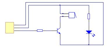
In this experiment, by programming the Raspberry Pi, we make the pin 11 of the Raspberry Pi output High and Low alternately, so the active buzzer makes sounds accordingly.
