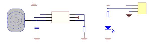
In this experiment, by programming the Raspberry Pi, we detect the High or Low of the output terminal of the Touch Button Module by pin 12 of the Raspberry Pi, so as to tell whether fingers touched the touch button or not.
