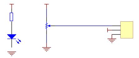
In this experiment, by programming the Raspberry Pi, we collect the analog values output by the Potentiometer module through pin CH0 of the ADC0832, convert it to digital values and display them on the terminal.
