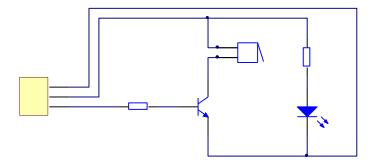
In this experiment, by programming the Raspberry Pi, we make the pin 11 of the Raspberry Pi output square waves of different frequencies alternately, thus driving the passive buzzer to play music.
