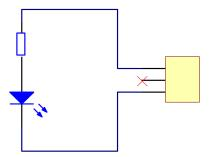
In this experiment, we make the pin 11 of the Raspberry Pi output High/Low by programming, to control the LED to blink in a certain frequency.
