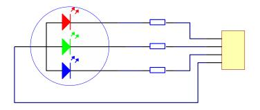
In this experiment, we make the pin 11, 12, and 13 of the Raspberry Pi output PWM (pulse-width modulation) signals by programming, to make the RGB LED flash different colors.
