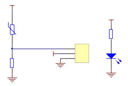
In this experiment, by programming the Raspberry Pi, we collect the analog values output by the Thermistor module through CH0 of the ADC0832, change it to digital values and display them on terminal.
