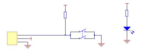
In this experiment, we detect the High or Low level of pin 12 of the Raspberry Pi and then control the LED connected to pin 11 accordingly.
