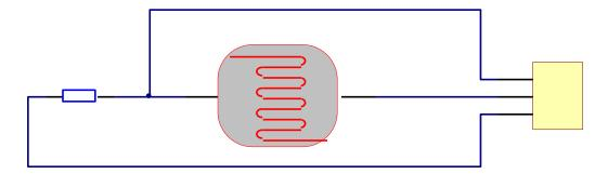
This experiment is to collect the data of light intensity by the Photoresistor module and then display it on the terminal.
