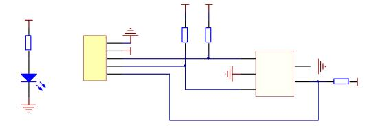
In this experiment, by programming the Raspberry Pi, we change a value by reading the status of the Rotary Encoder. When we turn the knob of the Rotary Encoder clockwise, the value on the terminal will increase; when we turn the knob counterclockwise, the value will decrease. When we press down the switch, the value will be zeroed out.
