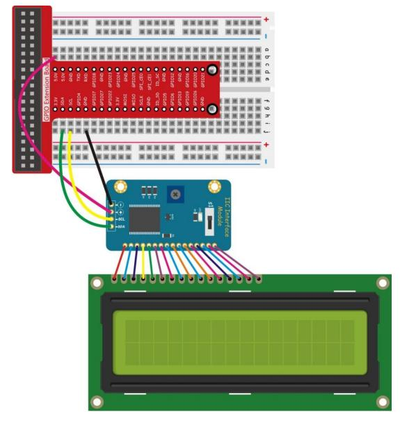
Step 2: The I2C of the Raspberry Pi is not turned on by default, we can use raspi-config to enable it
