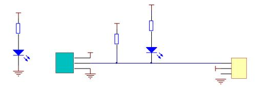
In this experiment, by programming the Raspberry Pi, we read the temperature value collected by the DS18B20 module through pin 7 of the Raspberry Pi, and display it on the terminal.
