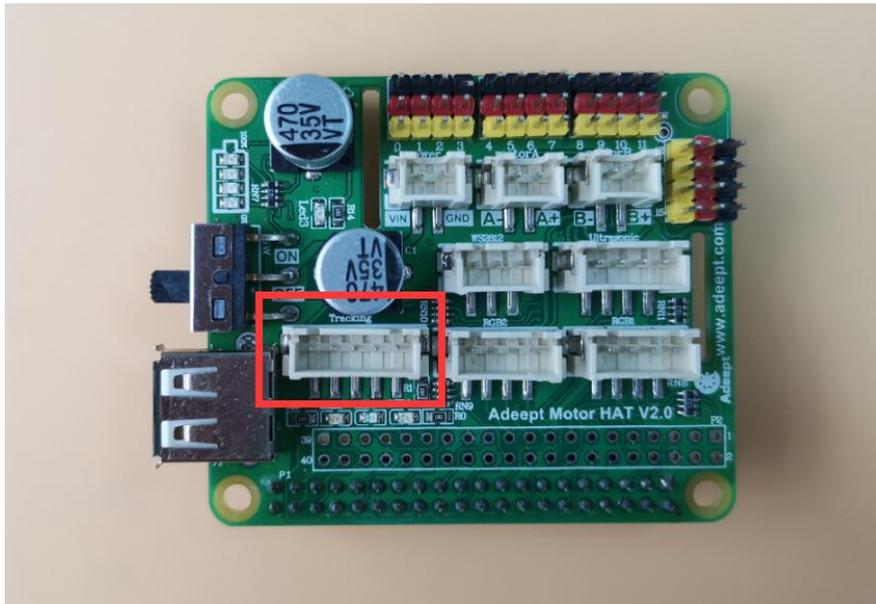
The pins of the three-way line inspection interface are from left to right: **3.3V**, **GPIO20**, **GPIO16**, **GPIO19**, **GND**.
