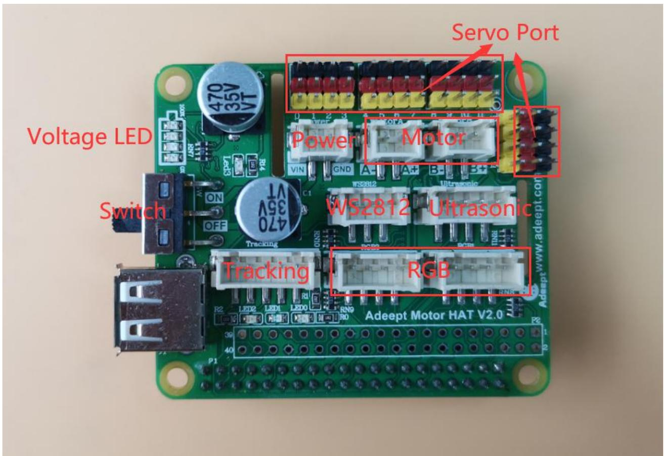
[Power]: The vin interface is an interface for external power supply.
