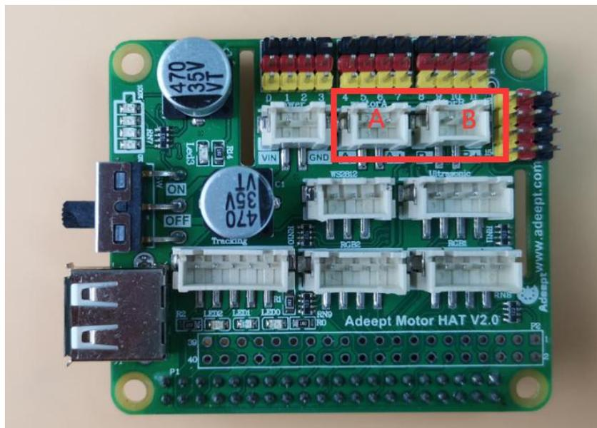
Two motor interface pins A and B, the left end of each interface is connected to the negative pole of the motor, and the right end is connected to the positive pole of the motor.
