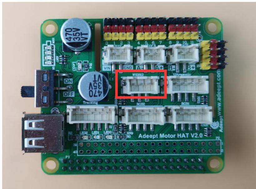
The ws2812 interface pins are from left to right: **GPIO12**, **5V**, and **GND**.
