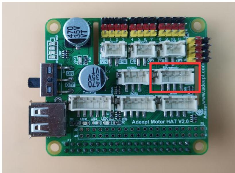
The ultrasonic interface pins are from left to right: **5V**, **GPIO11**, **GPIO08**, **GND**.
