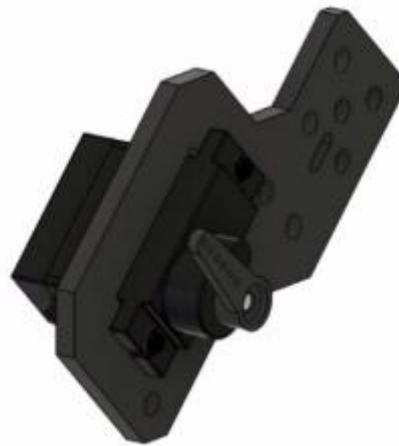
(2) Then use 2 M3x10 Screws and 2 M3 Nuts to install the disassembled A03 part (including the servo) to the side of L04, as shown in the following figure:
