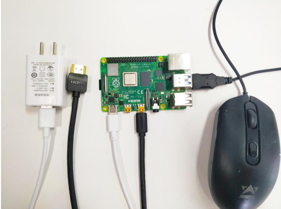
Connect the HDMI cable to the HDMI port of the monitor:
