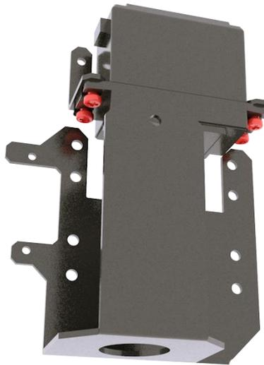
Use M3X4 screws to fix the servo to the servo bracket as shown in the two pictures above. The servo bracket has tapped threads, so no nuts are needed for installation here.
