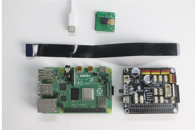
Install the camera cable, contact the metal surface of the cable with the metal surface of the Raspberry Pi (the same is true for installing the camera).
