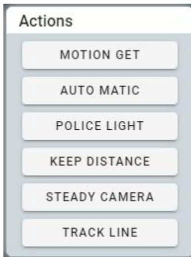
MOTION GET: switch watchdog mode. In this mode, the robot product stops moving and reacts to the moving objects detected in the camera. The moving objects are framed in the video of the Vedio module.
