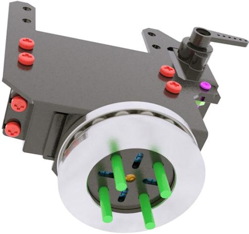
Install the 51105 thrust bearing. Note here that the thrust bearing consists of three separate parts. Subsequent assembly will compress the thrust bearing.
