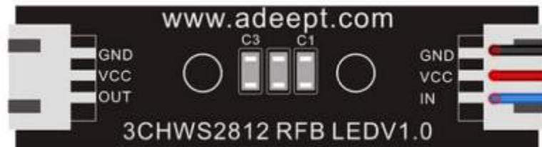
WS2812 LED light is a very commonly used module on our robot products. There are three WS2812 lights on each module. Please pay attention to the signal line when connecting. The signal line needs to be connected to WS2812 after being led out from the Raspberry Pi. At the "IN" end of the LED light module, when the next WS2812 LED module needs to be connected, the signal line is drawn from the "OUT" end of the previous WS2812 module and connected to the "IN" end of the next WS2812 LED.
