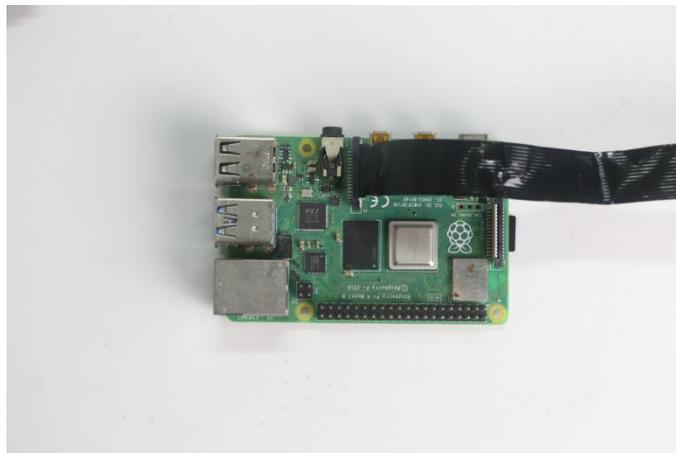
Install Robot HAT and camera, and connect the Raspberry Pi power supply.
