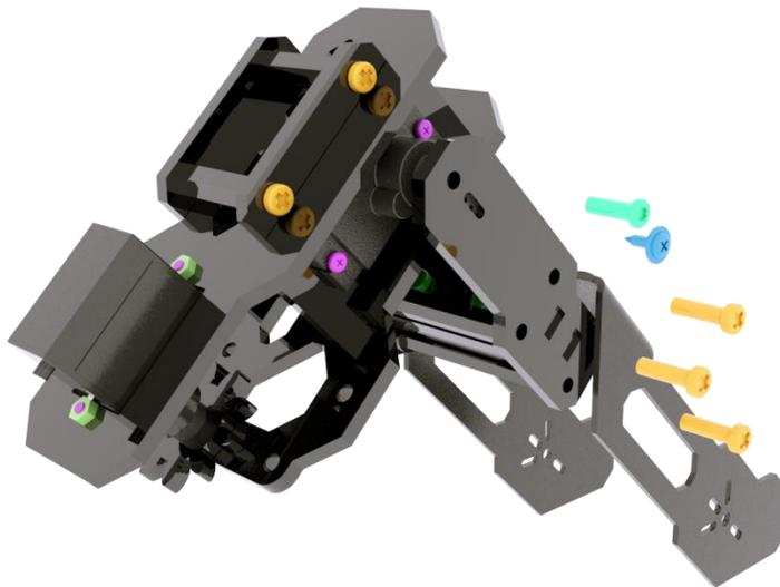
Use three M3X10 screws to fix the panel on the other side.
