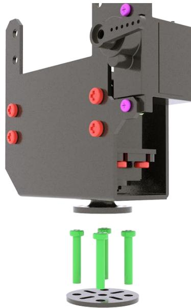
Install the round rocker arm of the large metal servo, and pierce the M3X16 screws through the round aluminum alloy parts shown below.
