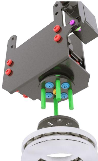
Then install a round aluminum alloy part, and then install 51105 thrust bearing.
