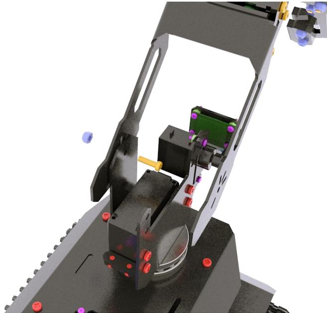
Use M3X10 screws and M3-LOCK lock nuts to fix the robot arm to the base of the PTZ.
