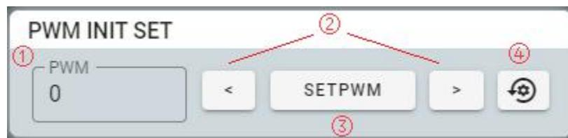
It is used to fine-tune the default angle of the servo, which can correct the angle error generated when the servo is installed. When returning to the center, the rudder will return to this default angle.
